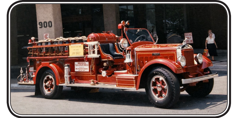
Hanover Fire Co. No. 1, 46-1 / Hanover, PA. 1935 MACK BX 75 open cab, 750 GPM pump, 100 Gallon Water. Transferred to Clearview Fire Co. No. 3, then to Hanover Borough Landfill, Bill Radish, Shane Graf and now in New England.
