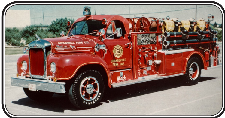
Grangeville / Goodwill Fire Co. 51 / Penn Twp. 1961 B1 MACK, semi open cab, 750 GPM Pump, 500 Gallon Water. Was involved in a vehicle accident at Blooming Grove Rd. and York St. Sold to private owner in Leesburg, VA.
