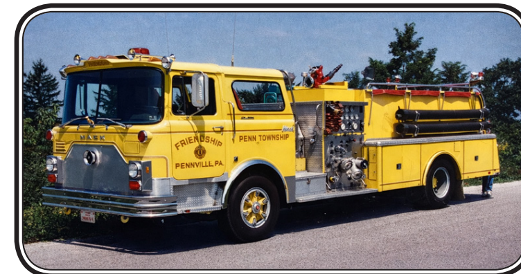
Pennville / Friendship Fire Co. 48 / Penn Twp. 1977 CF Mack, gas engine, 1,250 GPM Pump, 1,000 Gallon Water. Sold to Buddy Gray, Fire Apparatus dealer in Alabama.
