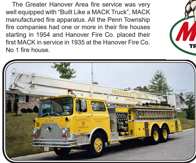
Pennville / Friendship Fire Co. 48 / Penn Twp. 1970 CF Mack, gas engine, 1,000 GPM Pump, 200 Gallon Water, 85 foot Snorkel.
