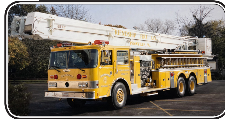
Pennville / Friendship Fire Co. 48 / Penn Twp. 1970 CF Mack remounted on 1989 Pierce Arrow chassis, 1,000 GPM Pump, 200 Gallon Water, 85 foot Snorkel. Sold to Ozark, MO then to Richmond, MO. Totaled in a rollover accident.
