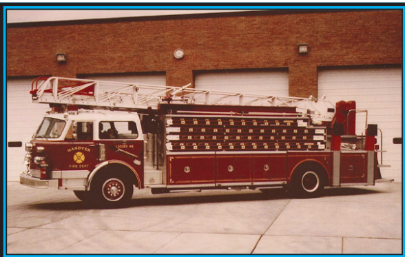
1977 1000 Series 100 Foot Rear-mount Aerial No Pump V-6 Detroit Wirt Park
