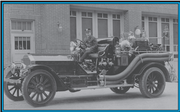
1917 Type 75 750 GPM 6 Cylinder Triple Combination Co. No. 2
