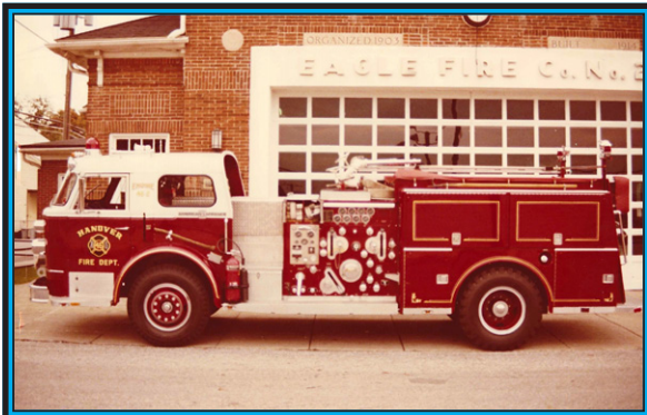
1970 Type 900 Series 1000 GPM 500 Gallons Water 6 Cylinder Co. No. 2
