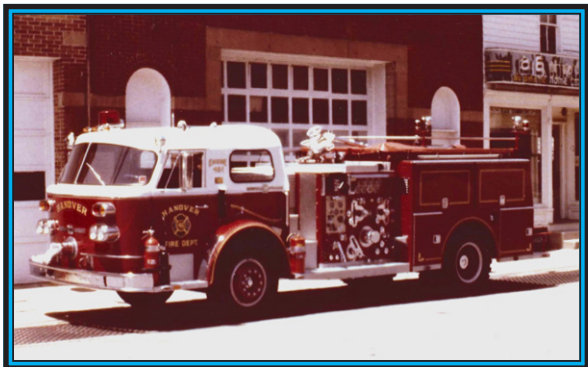
1970 Type 900 Series 1000 GPM 500 Gallons Water 6 Cylinder Co. No. 1
