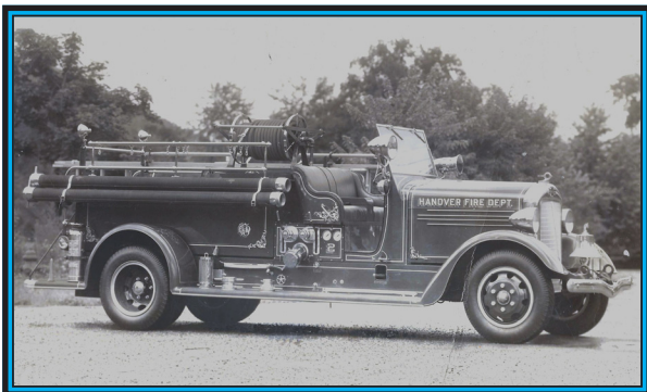
1937 Type 400 Junior 750 GPM Triple Combination 12 Cylinder Co. No. 2
